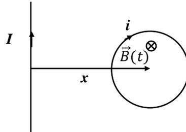
$$B(I) = \frac{\mu_0 I}{2\pi x} = \frac{\mu_0 I_0 \sin \omega t}{2\pi x} \Rightarrow \phi = f(t) \Rightarrow i \neq 0 = \frac{e}{R}$$
