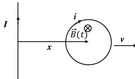
$$B(I) = \frac{\mu_0 I}{2\pi x} \text{ et } x = \text{cte} \Rightarrow \phi = \int B ds = \text{cte} \Rightarrow e = \frac{-d\phi}{dt} = 0 \Rightarrow i = 0$$
