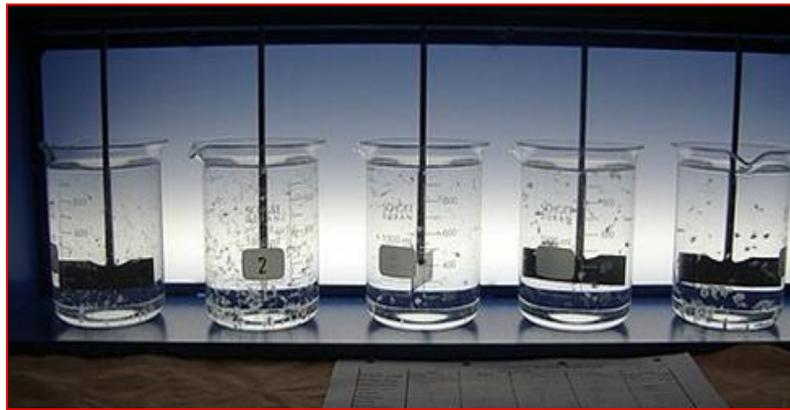
Figure II.3. Essai de coagulation Jar-test
