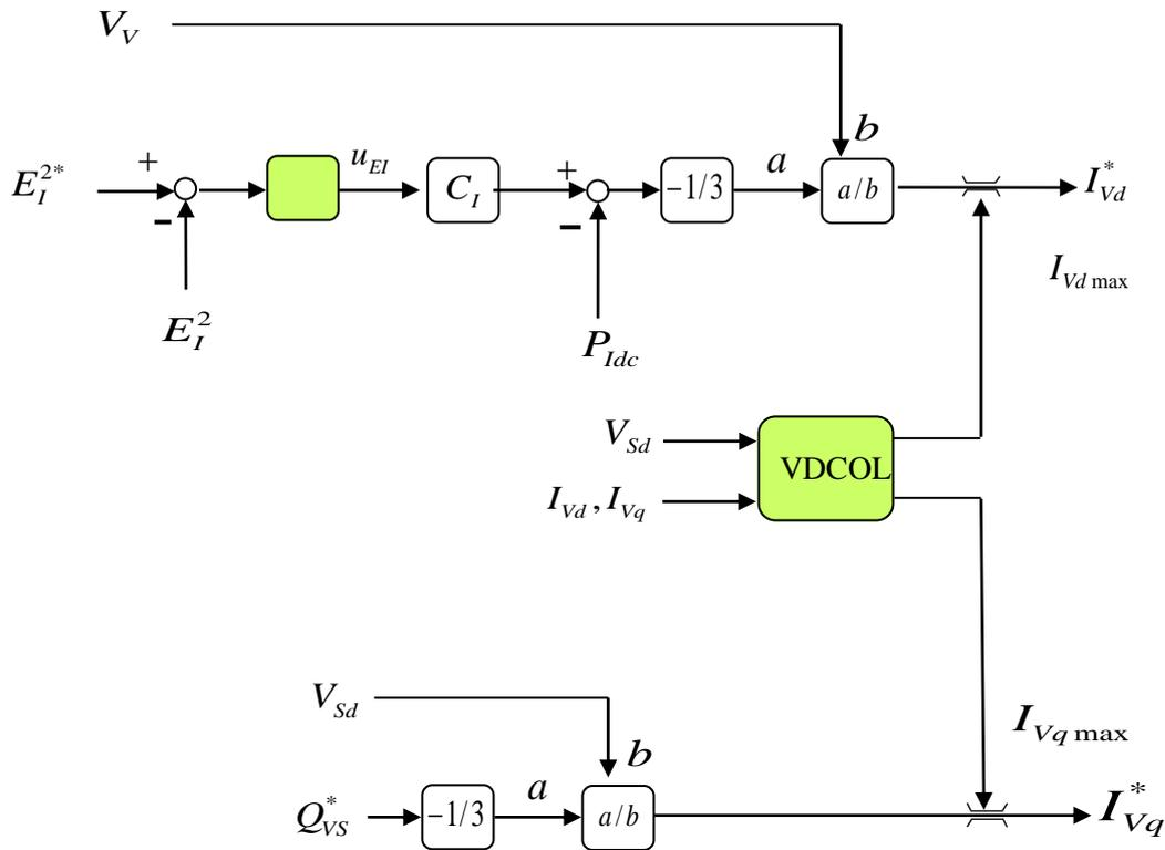
Fig. 4.22 : VSC converter external control block diagram
