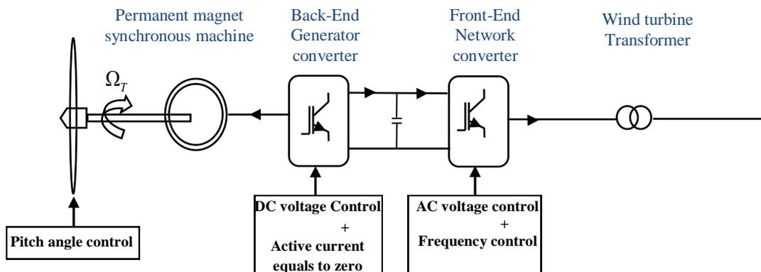
Fig. 4.17: Global Equivalent Offshore Wind Farm Control System
