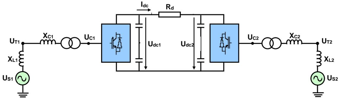
Fig. 2.6: Basic configuration of a point-to-point HVDC VSC link
