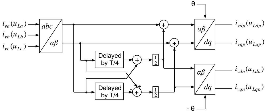
Fig. 3.3: Separation of positive and negative sequence components
