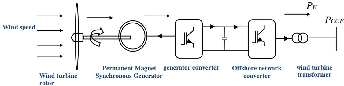
Fig. 4.6: Wind turbine components
