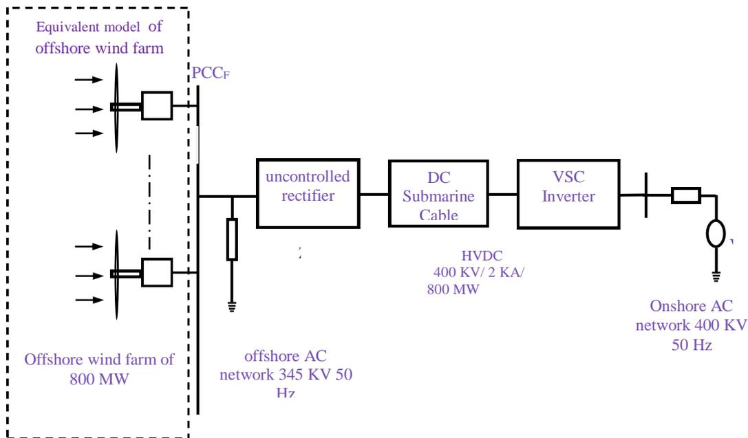
Fig. 4.2: The configuration of a wind farm connected to an HVDC system based on an uncontrolled rectifier and a VSC inverter
