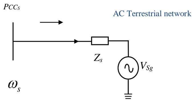
Fig. 4.15: Terrestrial Network Model
