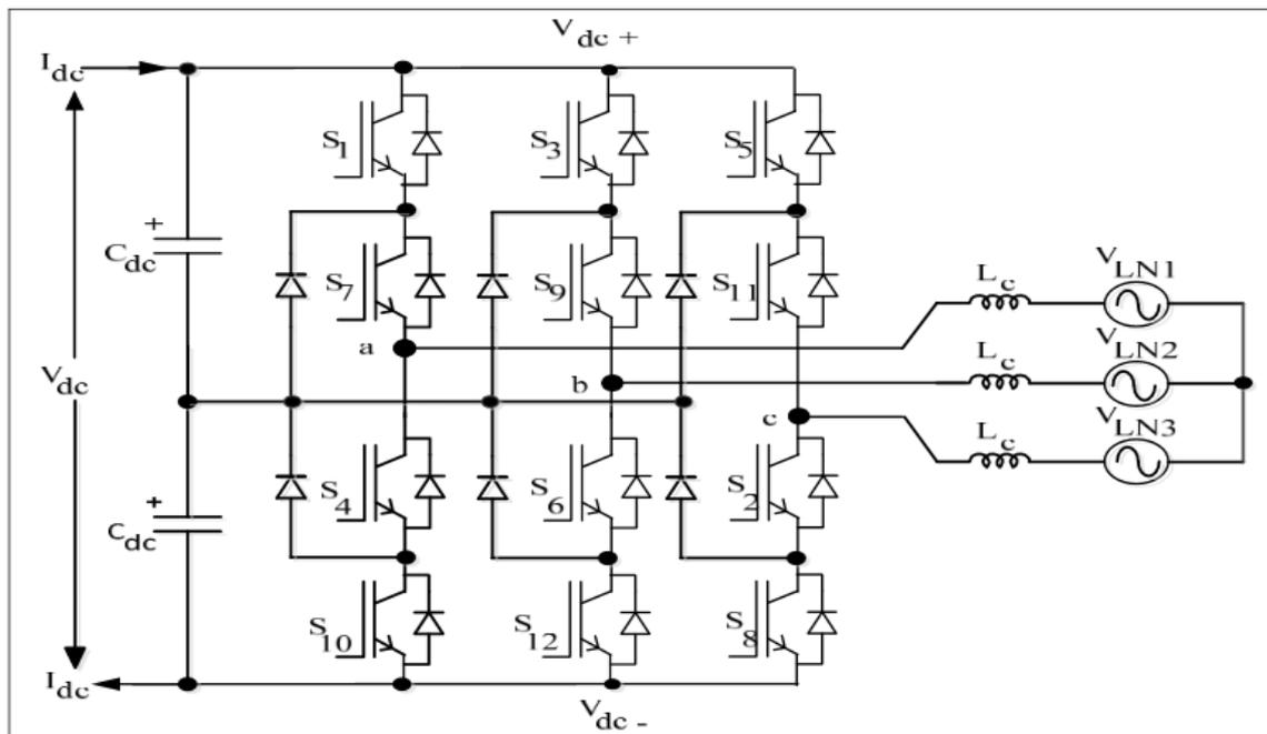
Fig.2.2: a three-level HVDC converter
