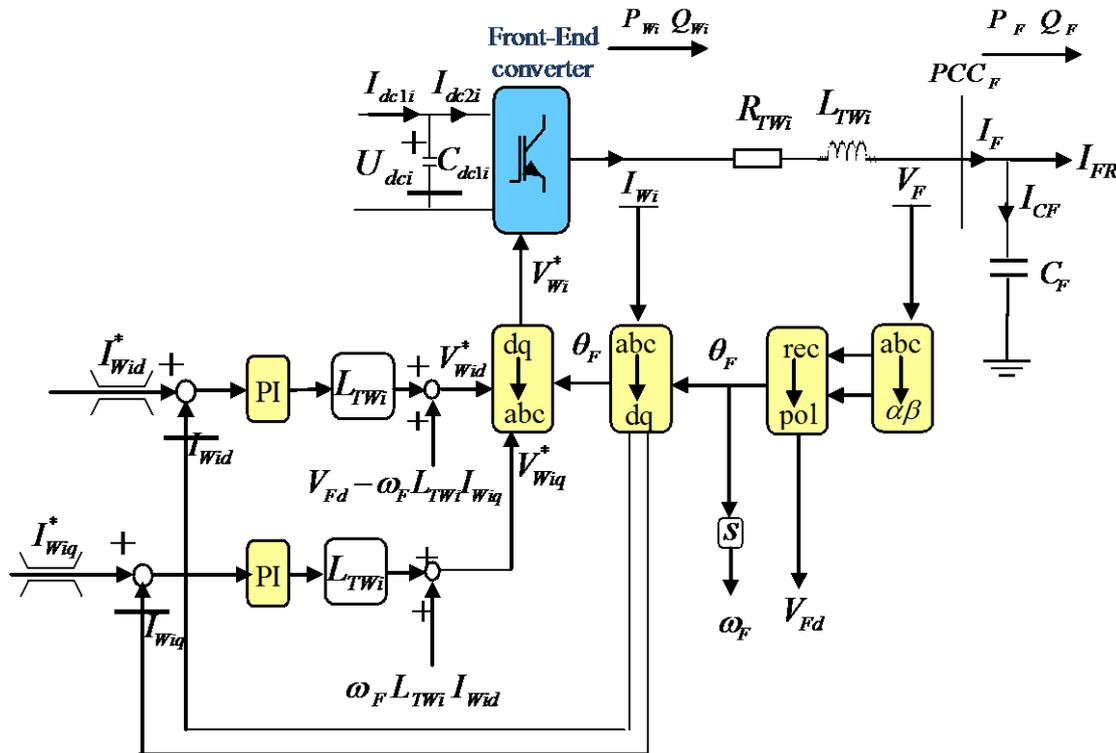
Fig. 4.19 : Current control block diagram
