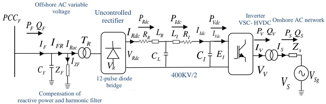
Fig. 4.7: HVDC transmission configuration
