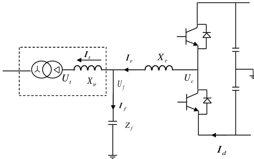
Fig. 4.12: Equivalent diagram of the VSC circuit
