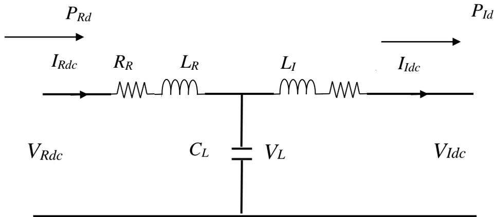
Fig. 4.9: Model of the submarine "T" cable
