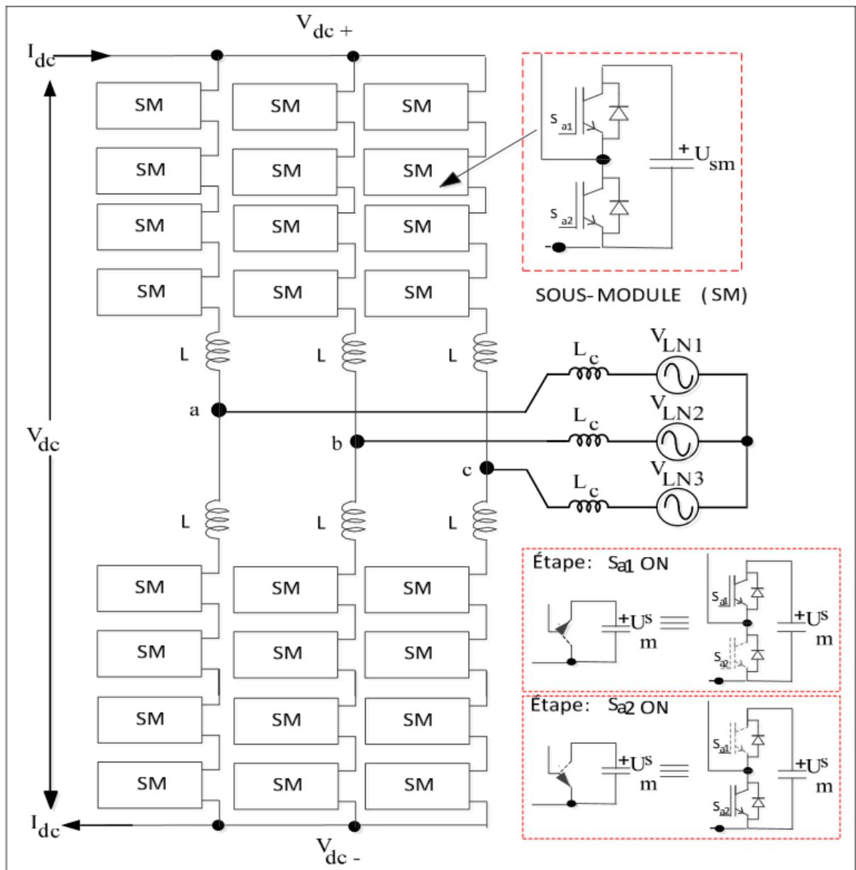
Fig.2.3: The three-phase Multilevel Modular Converter
