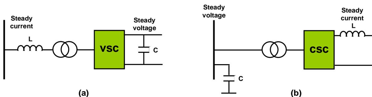
Fig. 2.10: (a)- Self Commutated Voltage Source Converter (VSC)
