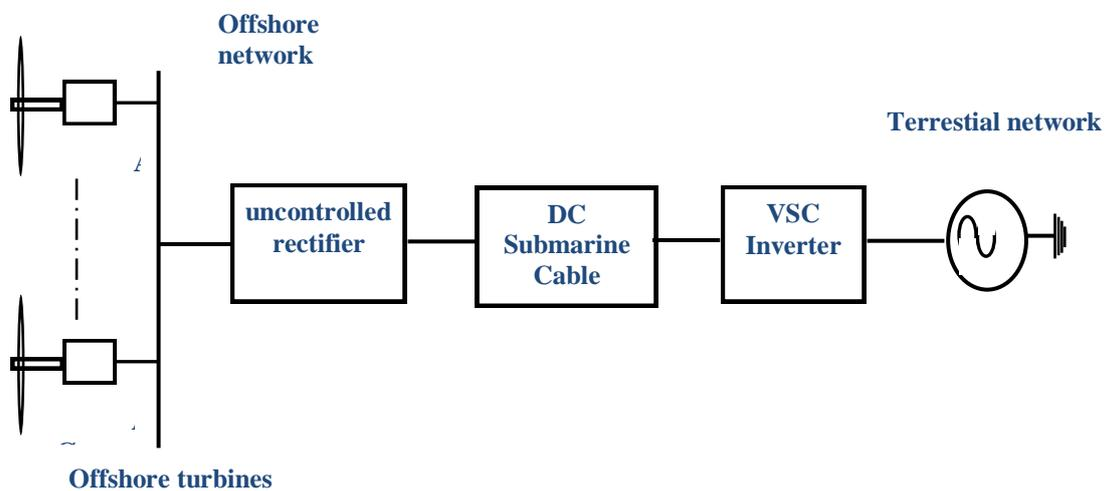
Fig. 4.1: Offshore wind farm connected to HVDC system of uncontrolled rectifier and VSC inverter
