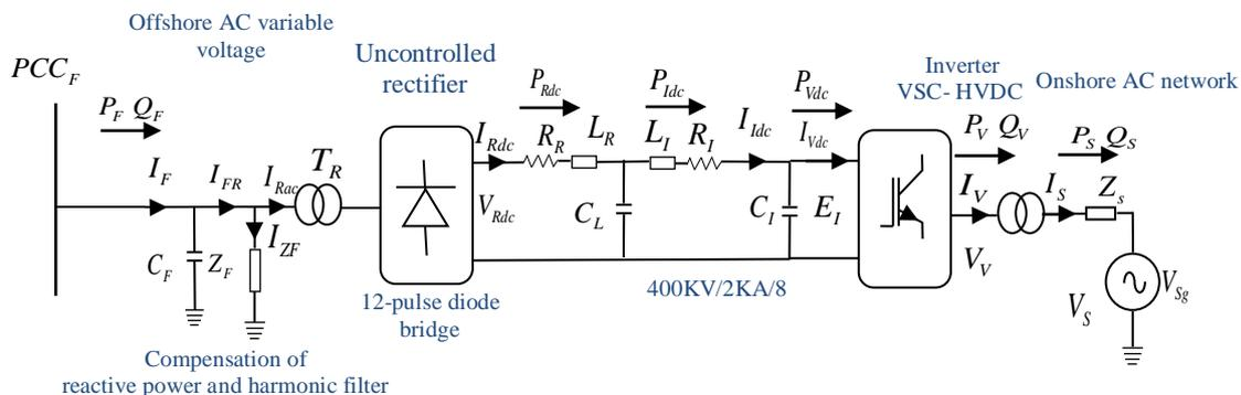
Fig. 4.5: Transmission HVDC-(Diodes - VSC)
