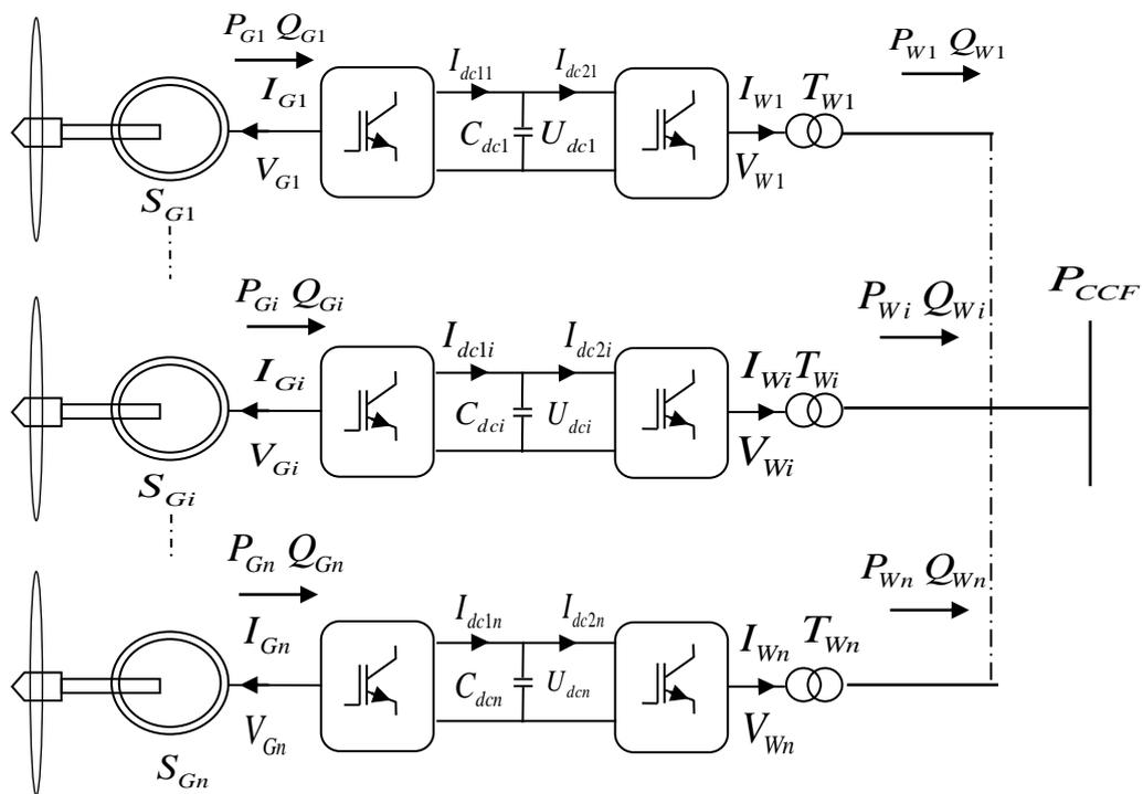
Fig. 4.4 : Offshore wind farm ( $i = 1,2,3,4,5$ ) connected to point  $PCC_F$
