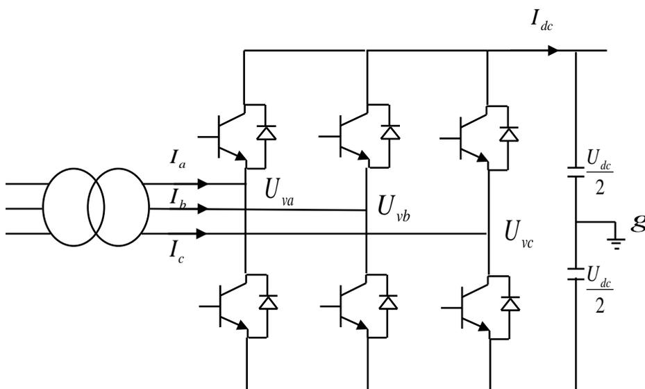
Fig. 4.10: Basic VSC circuit layout
