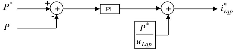
Fig. 3.6 : Control of active power
