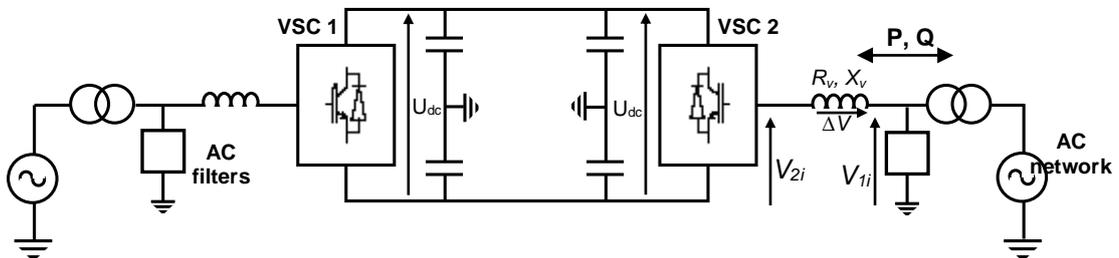
Fig. 3.9: Topology of a VSC-HVDC link
