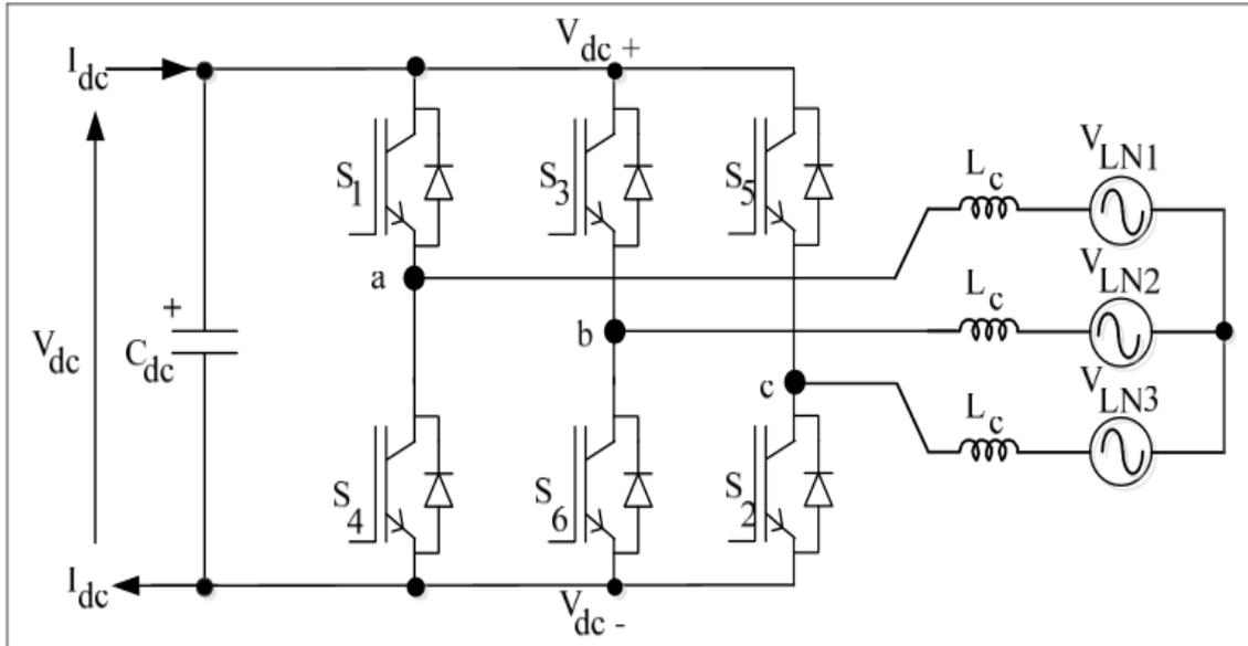
Fig 2.1: two-level HVDC converter
