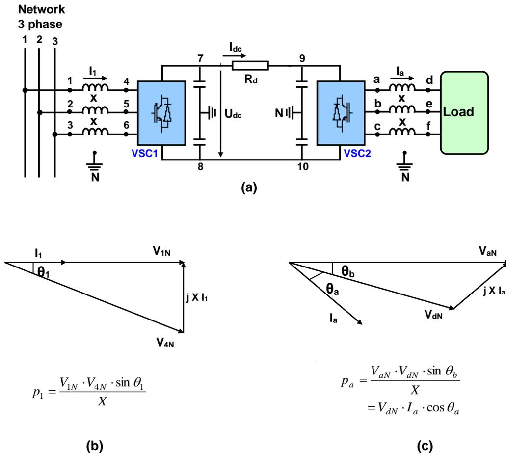
Fig. 2.9: (a)- Overview of a VSC-HVDC link feeding a passive network. (b)- Network side vector diagram. (c)- Vector diagram at the site.
