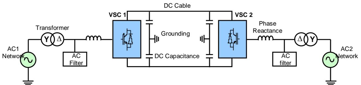
Fig. 2.4 : Components of a VSC-HVDC link
