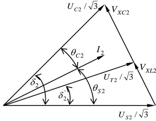
Fig. 2.8: Inverter side vector diagram
