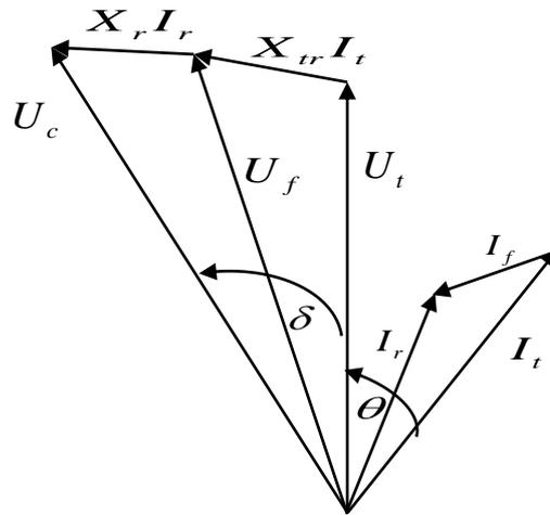
Fig. 4.13: Vector Representation of the VSC Circuit
