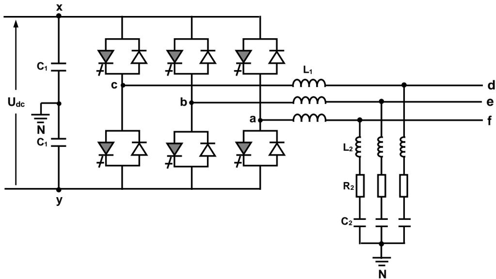
Fig. 2.5 : Composition of a conversion unit powered by a direct current source
