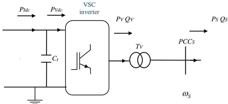
Fig. 4.14: VSC Terrestrial Inverter
