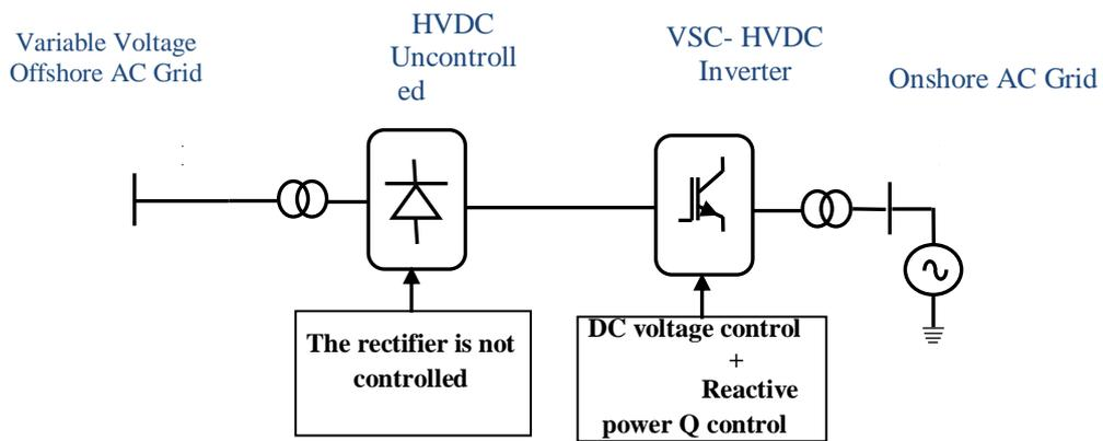
Fig. 4.16: HVDC-(Diodes-VSC) Overall Transmission Control System
