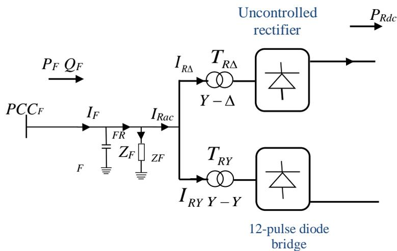
Fig. 4.8: Uncontrolled rectifier, capacitor, filter bank, and transformers
