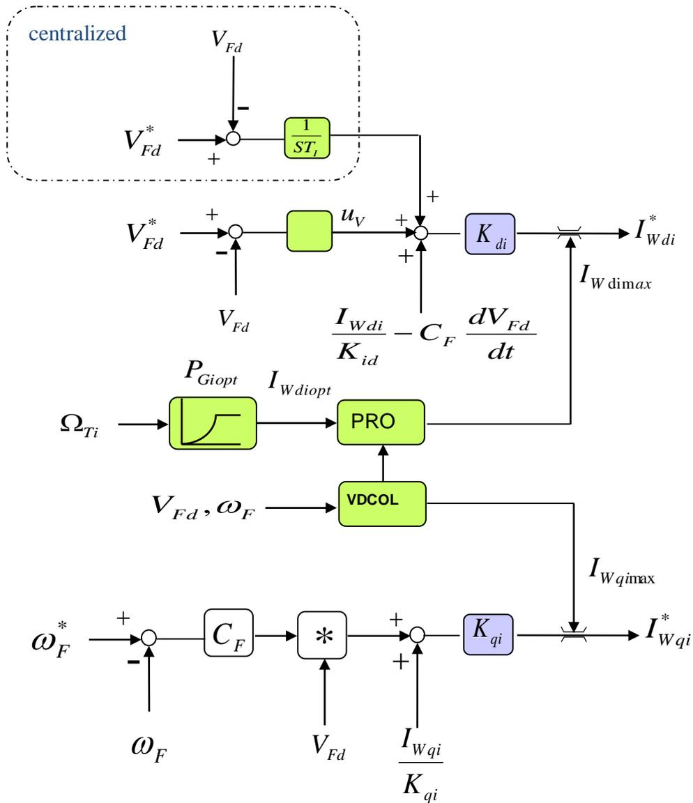
Fig. 4.20: Offshore Grid Voltage and Frequency Control Diagram
