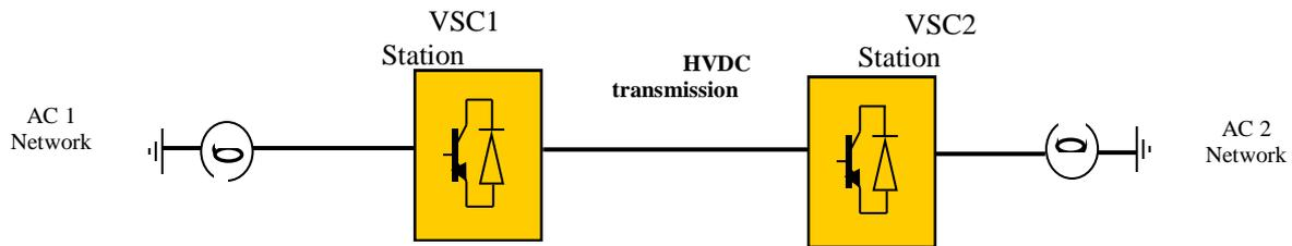
Fig.1.1: The description of VSC-HVDC transmission
