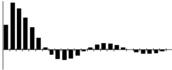
Figure 2.4. Example: Discrete unilateral frequency spectrum of the pulse.
