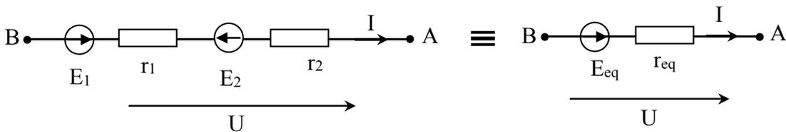
$$\Rightarrow \begin{aligned} E_{eq} &= E_1 - E_2 \\ r_{eq} &= r_1 + r_2 \end{aligned}$$
