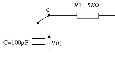
$$U_1 = U(t = 10 \text{ s}) = 10 \left( 1 - e^{-\frac{10}{2}} \right) = 9.93 \text{ V}$$
