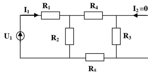
$$\boxed{R_{eq} = R_1 + \frac{R_2 (R_3 + R_4 + R_5)}{R_2 + R_3 + R_4 + R_5} = Z_{11}}$$
